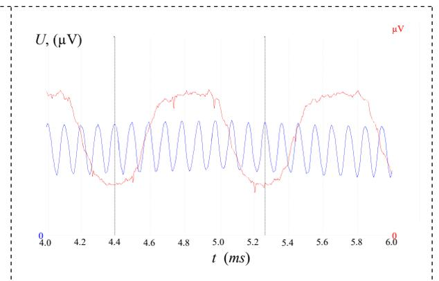
**Figure 4.** The signals of both reference encoder and a disk under test (lower frequency).
