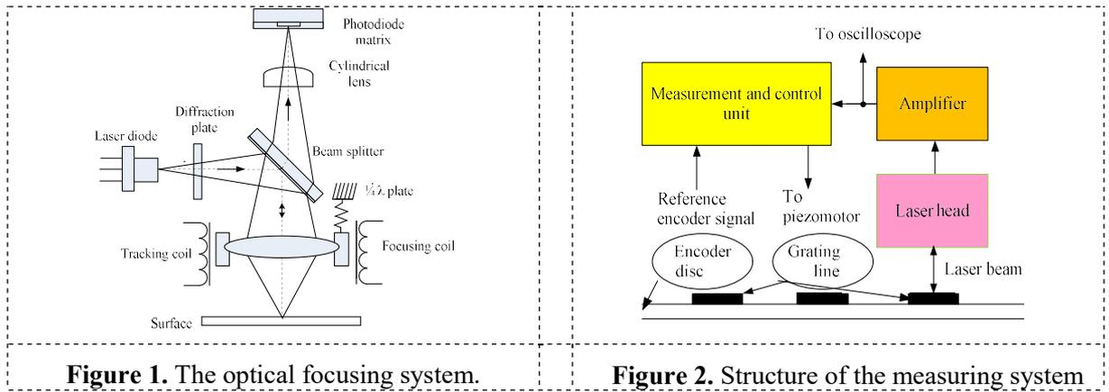
**Figure 1.** The optical focusing system.
