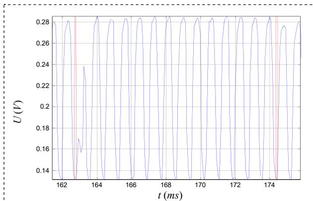
**Figure 3.** Signal of the disk grating with defects
